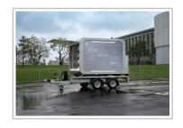
Mobile battery storage system BESS (Battery Energy Storage System) from JLR.
