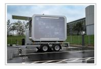
Mobile battery storage system BESS (Battery Energy Storage System) from JLR.
